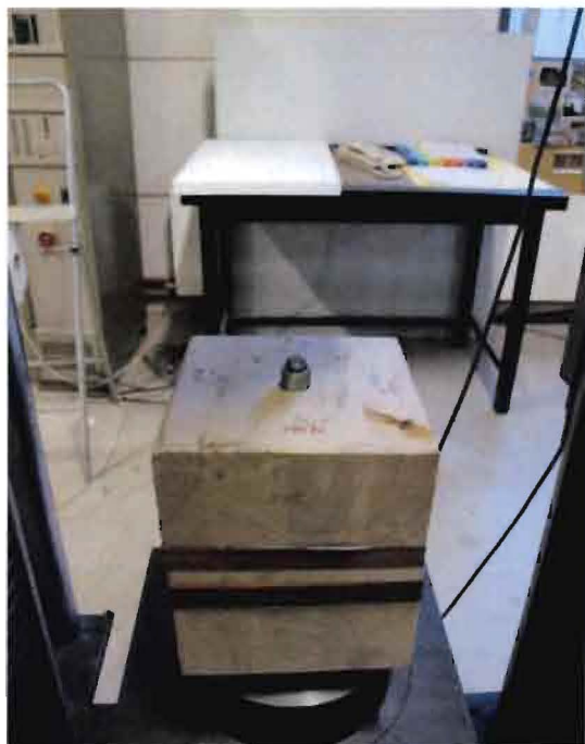
Figure 65 (left): Placement of members to connect on top of the tempex
