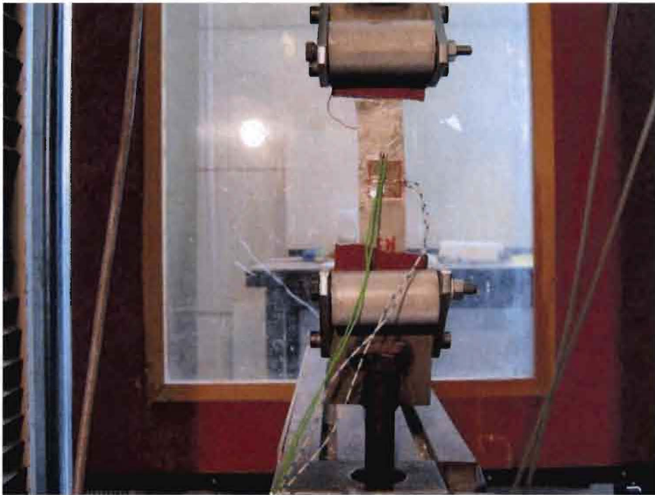
Figure 147: Adhesive failed due to tension (sample R3)
