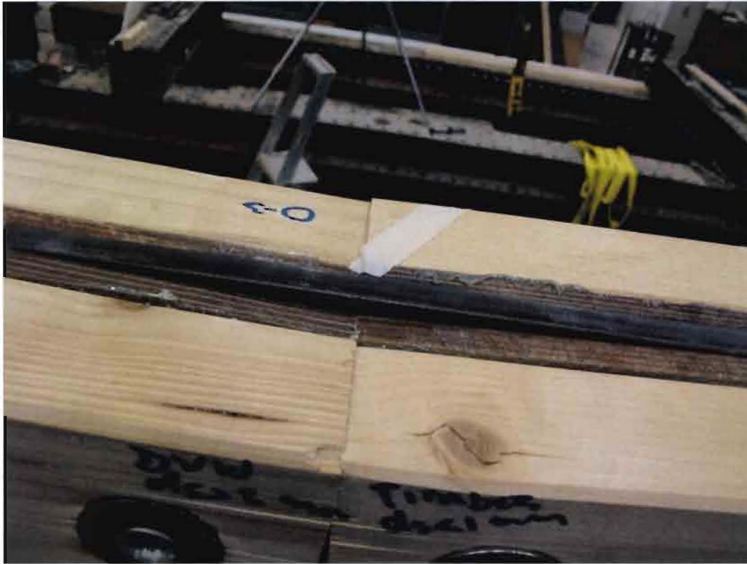
Figure 96: Compressed zone due to gap closure (sample 0-3)
