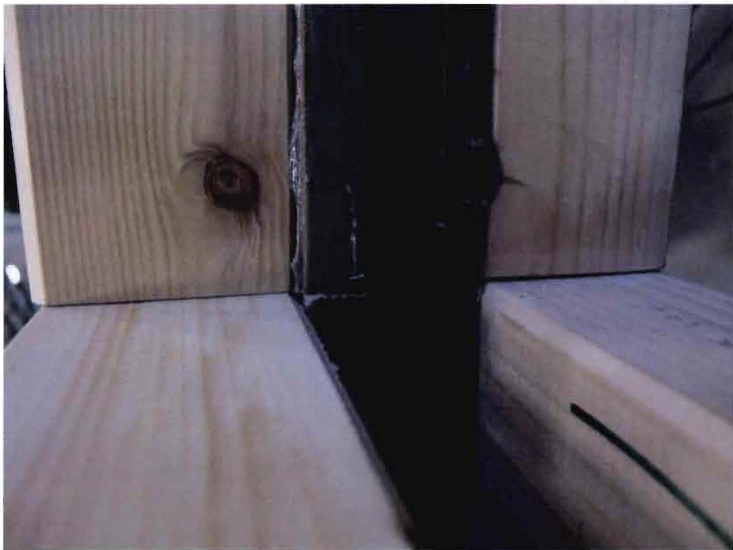
Figure 110: Close-up of gap before force initiation (sample 90-2)
