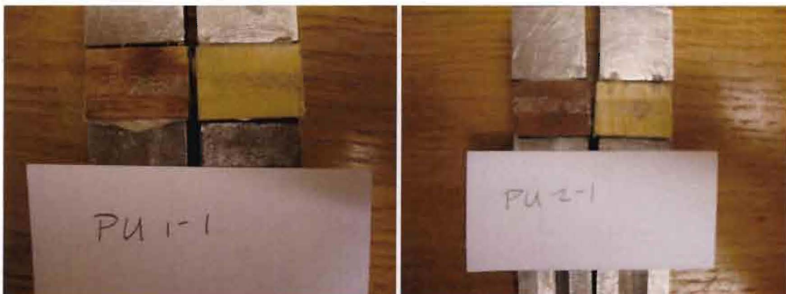
Figure 181: Results of shear tests with PU-based adhesive. d=0.1 mm; t > 4 days
