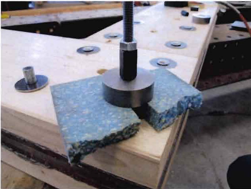
Figure 74: Placement of foam as distance holder
