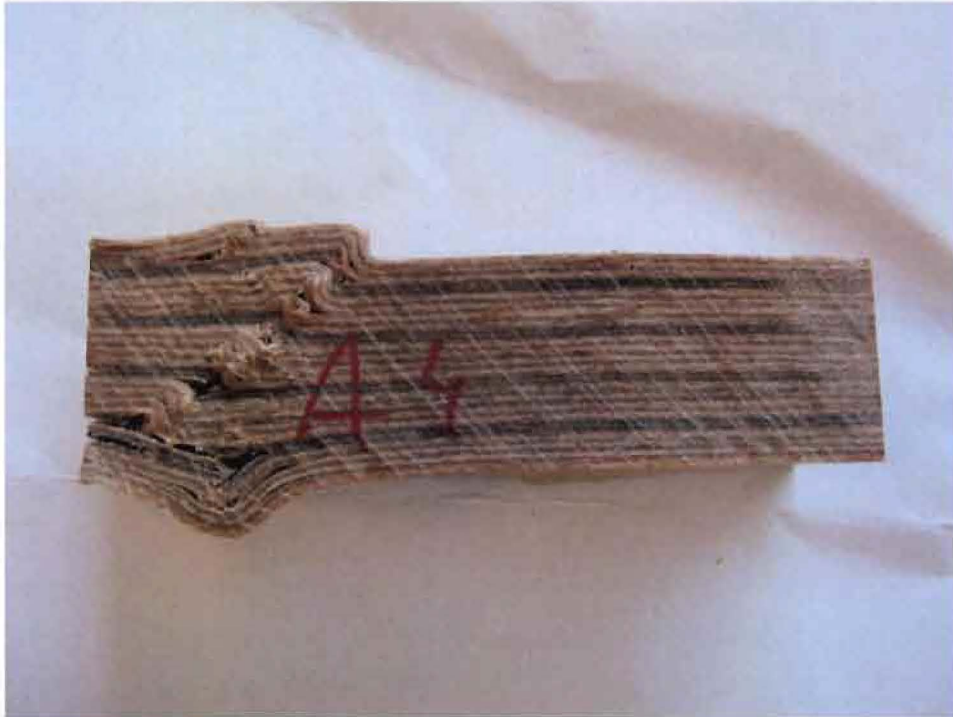
Figure 141: Failed dwv due to compression (sample A4)
