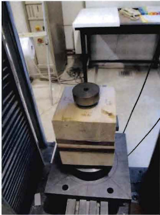
Figure 67 (left): Placement of upper mold
