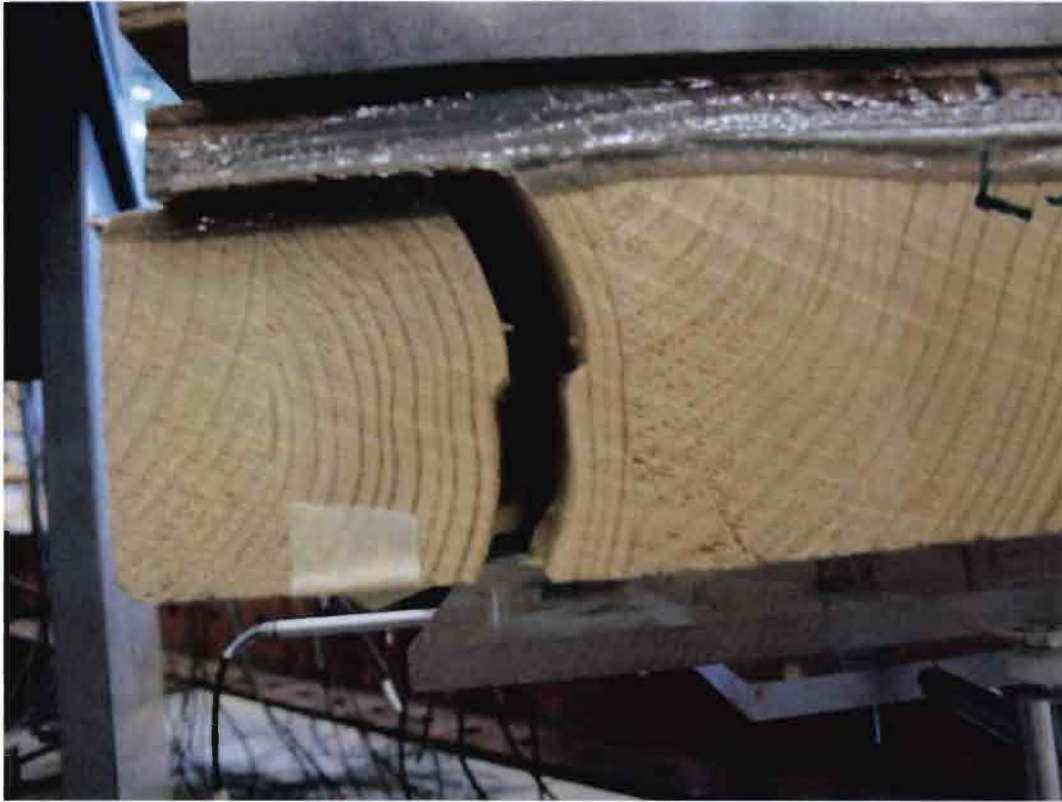
Figure 131: Failed connection (sample 90-4)
