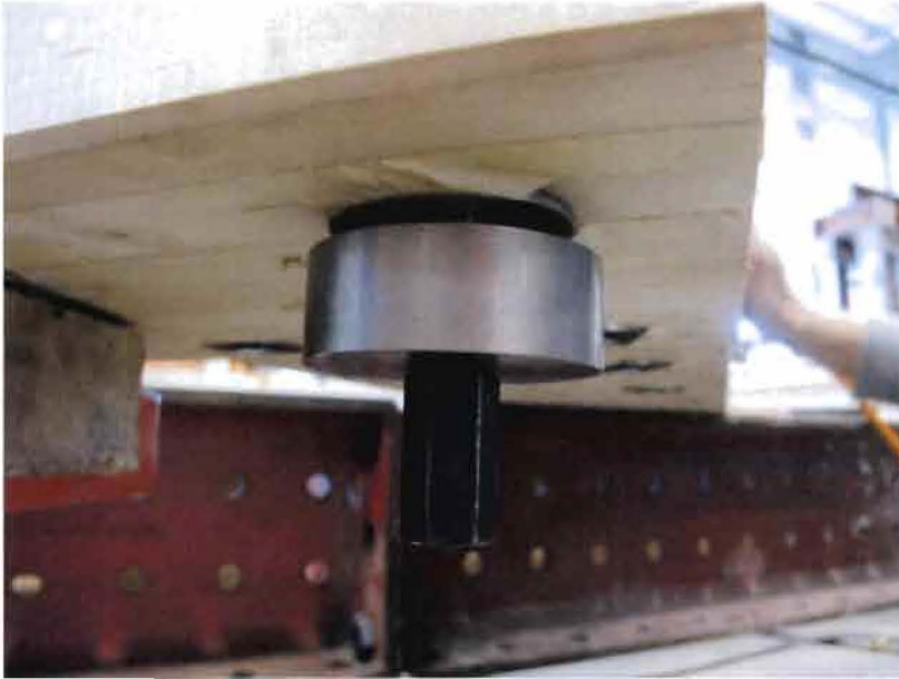
Figure 75: Placement of lower mold and nut
