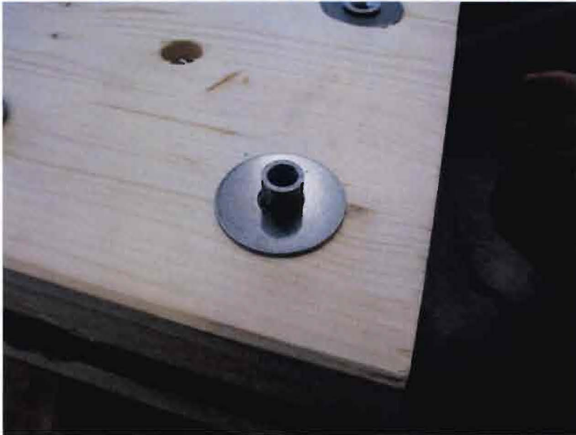
Figure 71: Placement of the tube and upper ring
