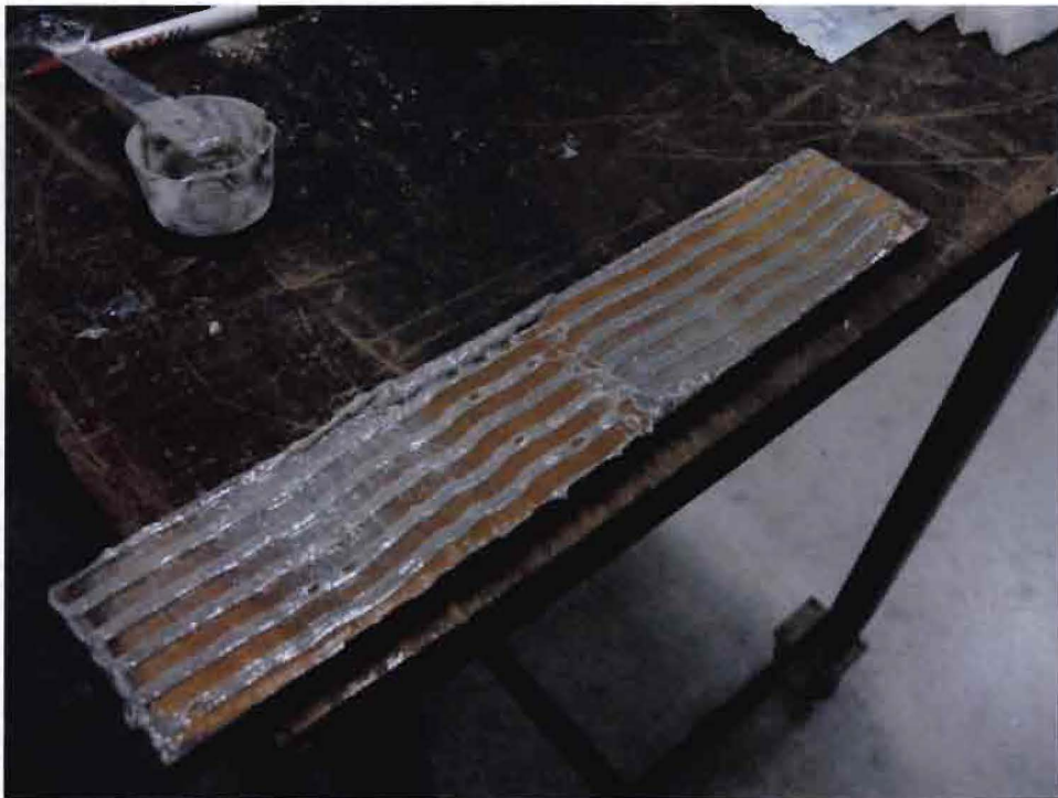
Figure 58: Surface glued by using a comb.
