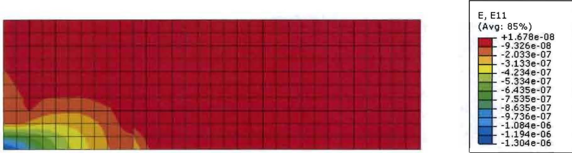
Figure 13: Strain in dwv and timber (back) with h_c/h= 0.2 and \Delta l=2.3911E-04 mm
