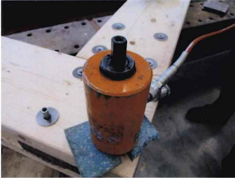
Figure 77: Placement of nut for fastening the rod to the hydraulic jack
