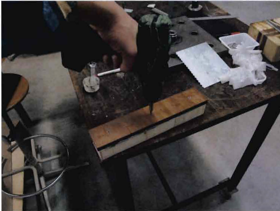
Figure 59: Screws as clamps
