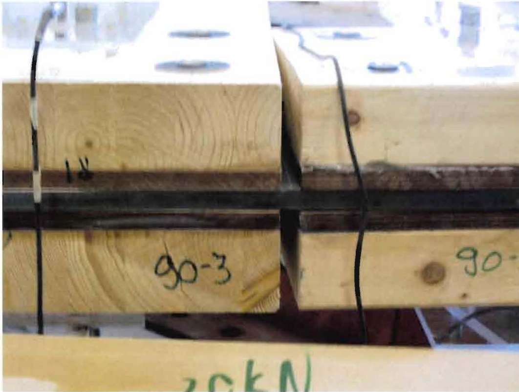
Figure 125: Gap; M = 38.2\text{kNm} (sample 90-3)
