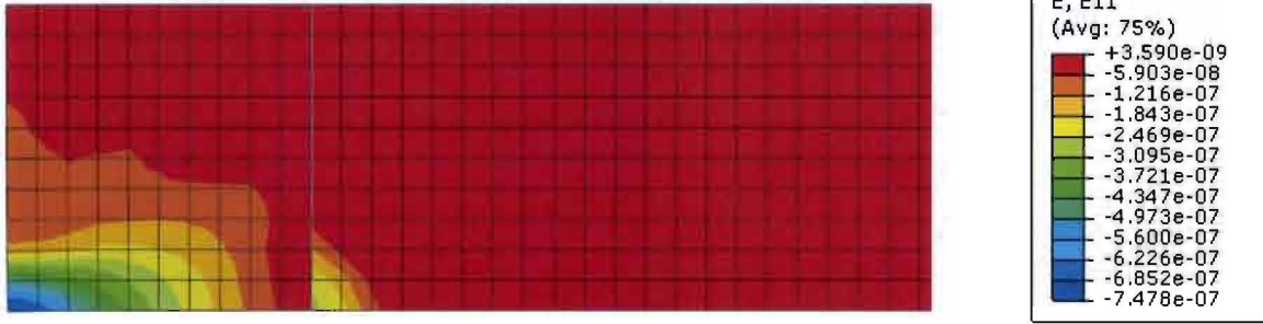
Figure 15: Strain dvw and timber (back) with h_v/h = 0.3 and \Delta l = 1.4980E-04 mm
