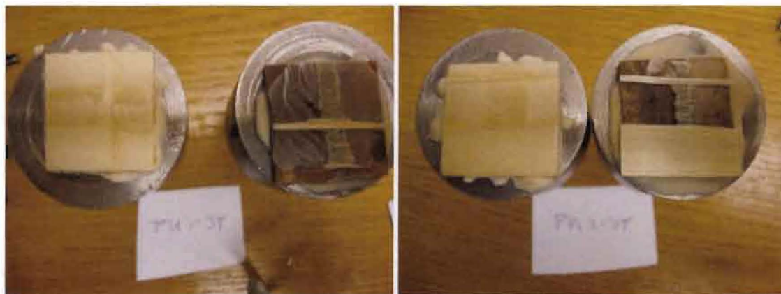
Figure 192: Results of tensile tests with poly-urethane based adhesive. d=0.3 mm
