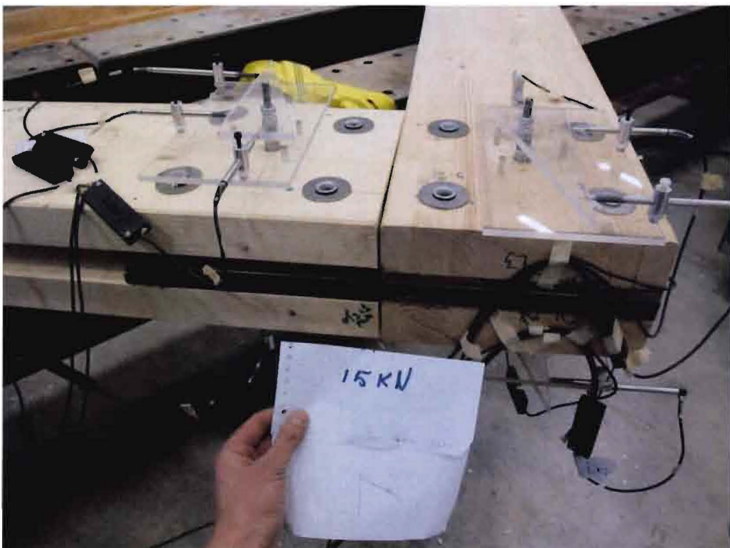
Figure 114: Connection with a bending moment of 28.6\text{ kNm} (sample 90-2)
