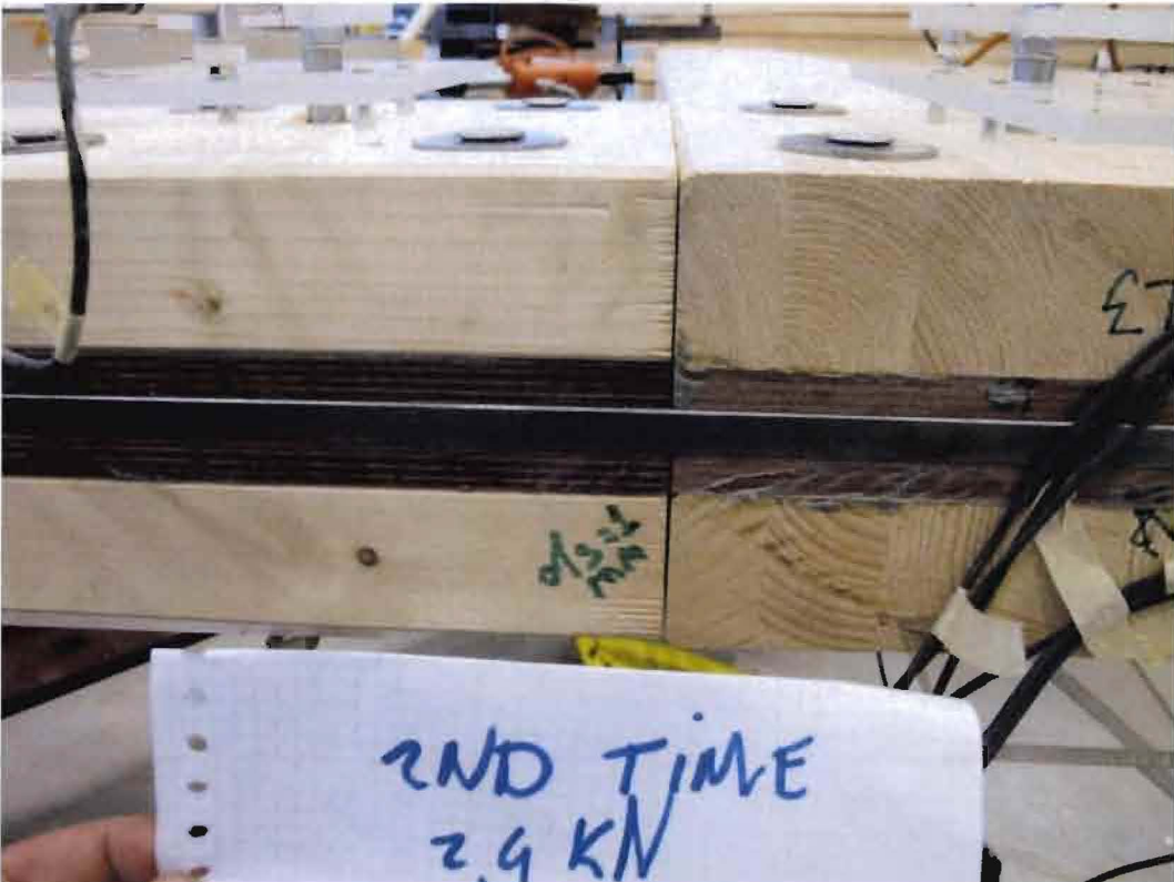
Figure 112: Gap after force diminishing; M = 4.6\text{kNm} (sample 90-2)
