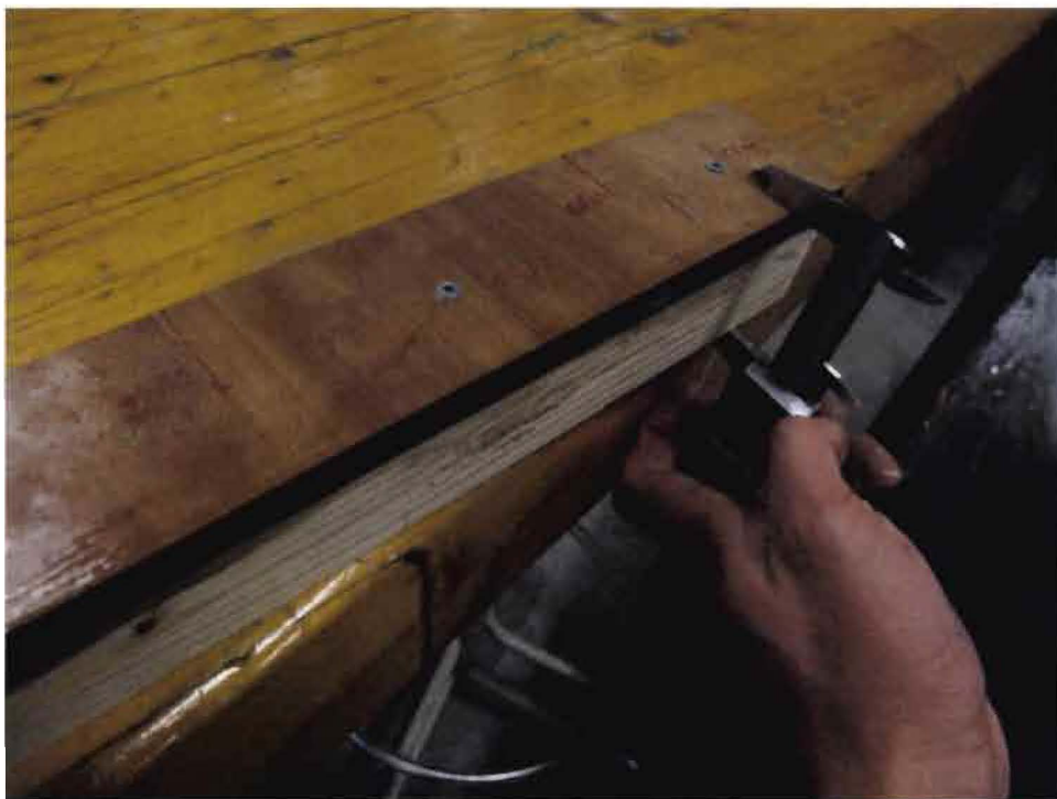
Figure 60: measurement of member thickness after gluing
