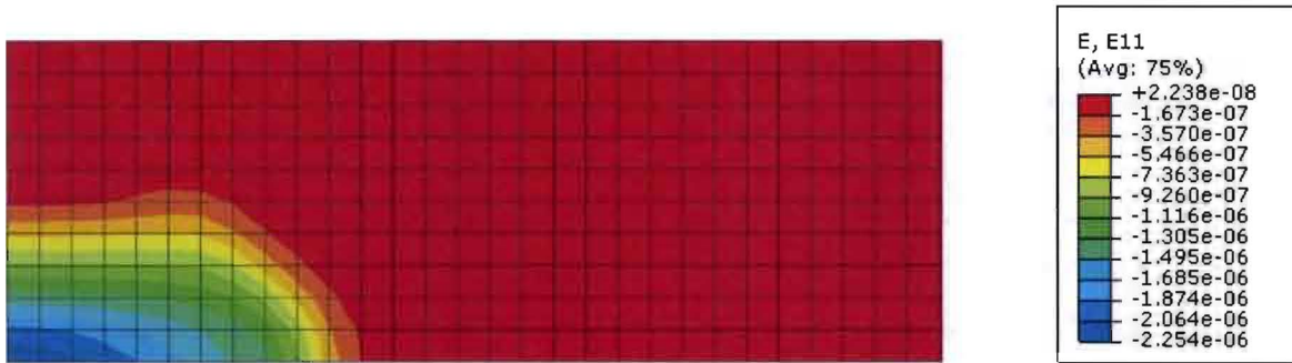
Figure 18: Strain timber with h_c/h= 0.5 and \Delta l=5.7500E-04 mm
