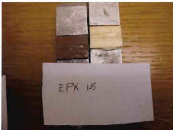
Figure 190: Results of shear tests with epoxy-based adhesive. d=0.5 mm
