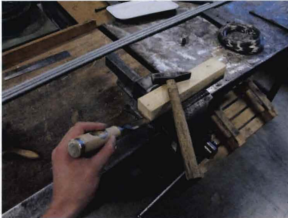
Figure 61: Separation of adherents
