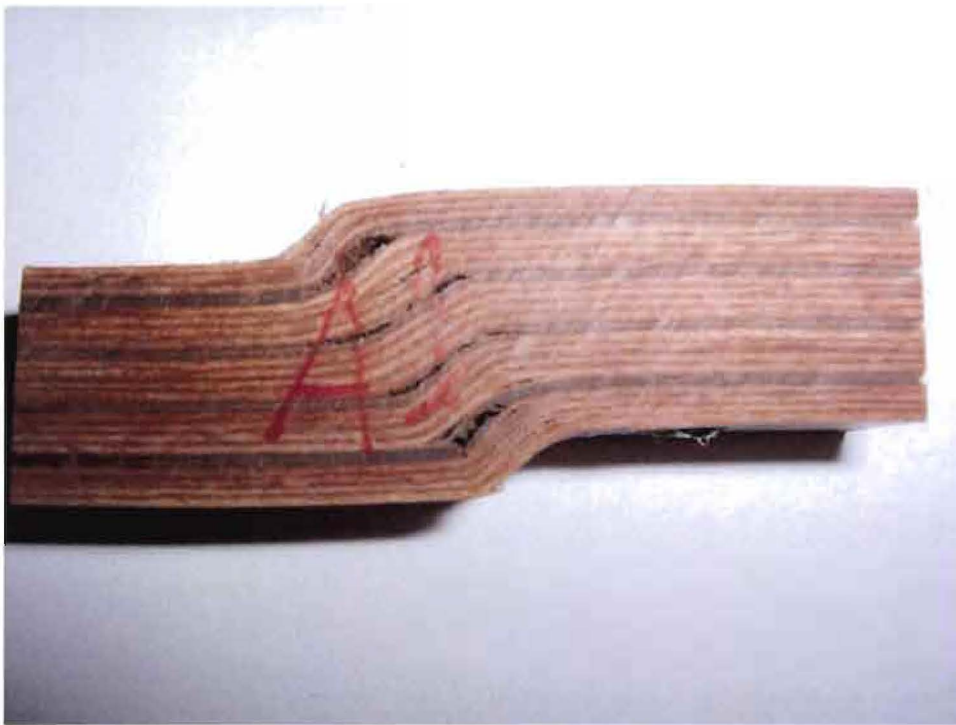
Figure 138: Failed dvw due to compression (sample A1)
