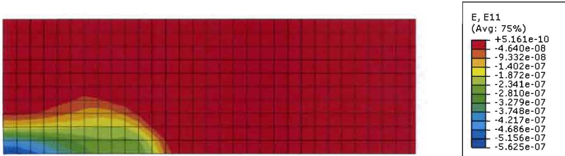
Figure 16: Strain timber with h_v/h = 0.3 and \Delta l = 1.4980E-04 mm
