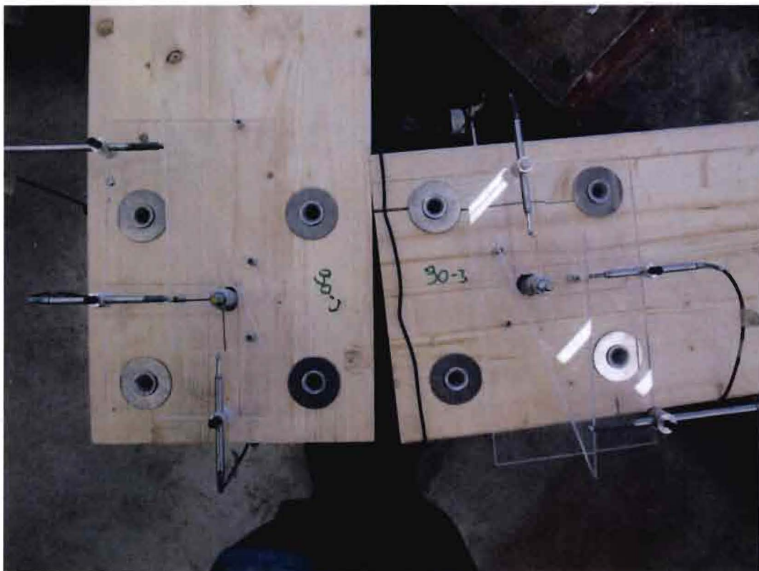
Figure 126: Failed connection (sample 90-3)
