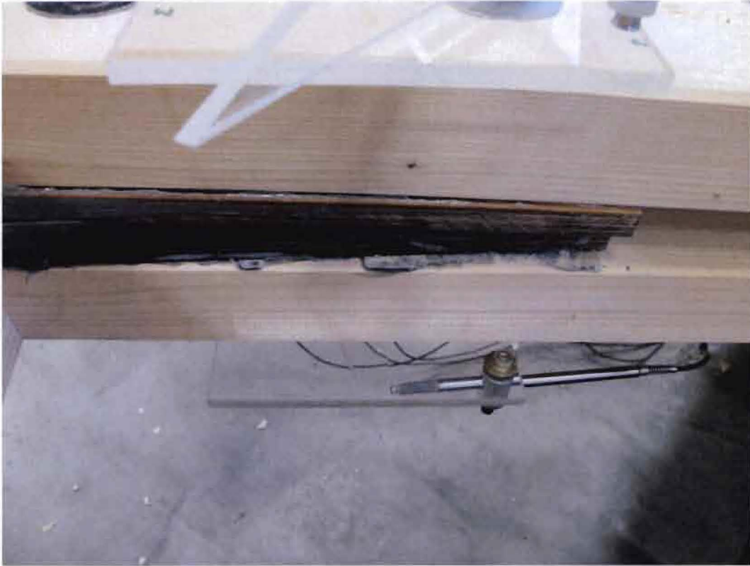
Figure 115: Failed bond line (sample 90-2)
