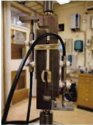
Figure 168: Shear tests set-up.
