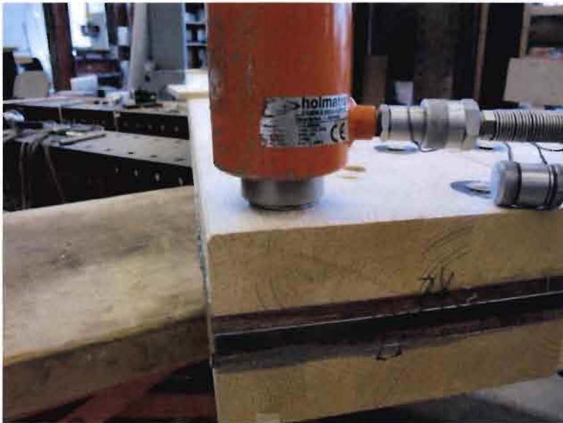
Figure 80: Removal of distance foam when hydraulic jack starts to move down
