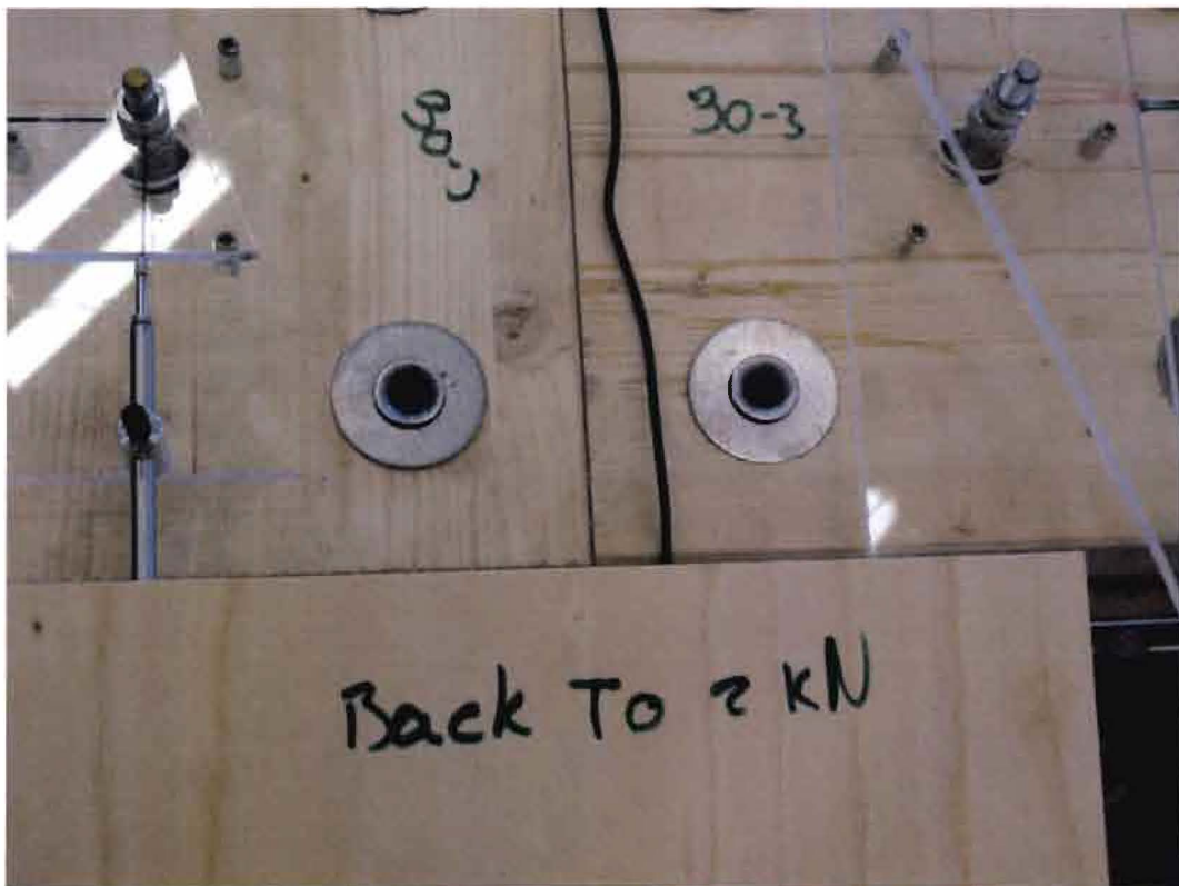
Figure 122: Gap after force diminishing; M = 3.82\text{kNm} (sample 90-3)
