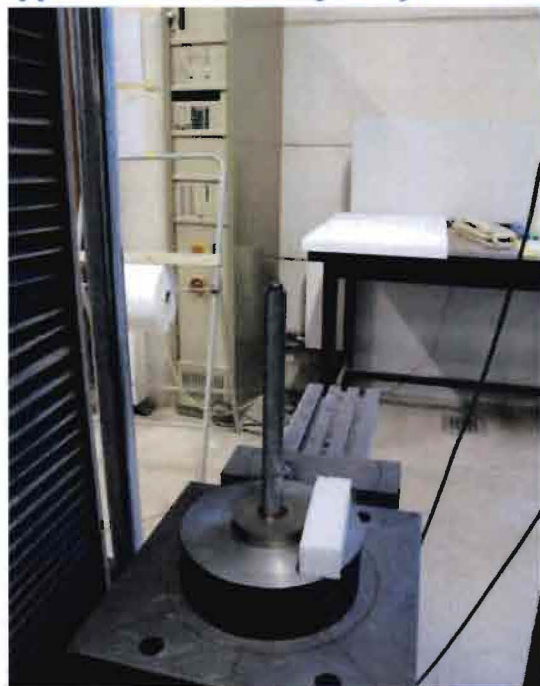
Figure 63 (left): Tube placed over rod that is placed in mold, tempex placed as support
