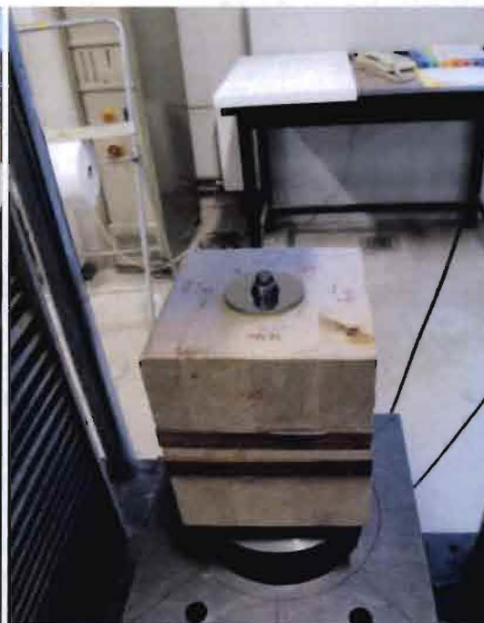
Figure 65 (left): Placement of members to connect on top of the tempex
