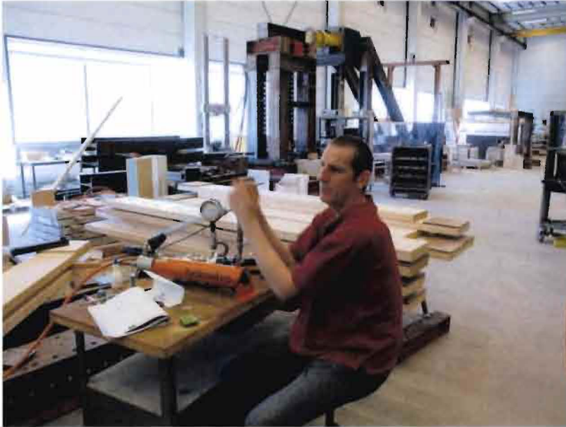
Figure 79: T.J.van de Loo increasing the tensile force up to 85-90kN (for 18mm tubes)
