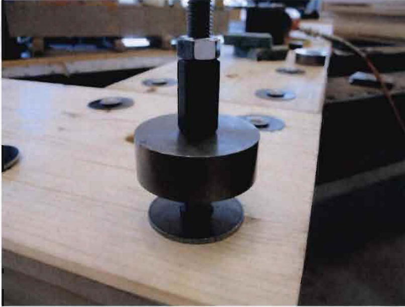
Figure 73: Placement of upper mold and (high capacity) threaded rod and nut
