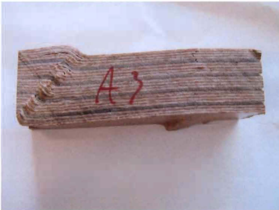
Figure 140: Failed dw due to compression (sample A3)
