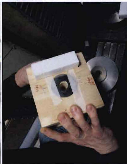
Figure 63 (left): Tube placed over rod that is placed in mold, tempex placed as support
