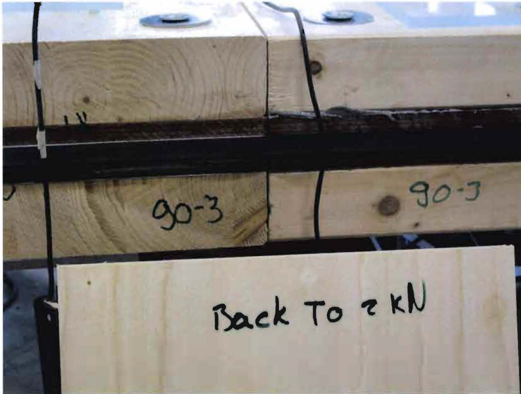
Figure 121: Gap after force diminishing; M = 3.8\text{kNm} (sample 90-3)
