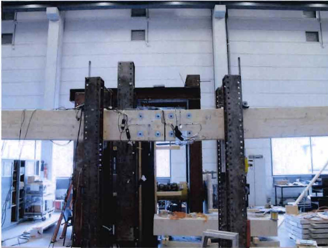
Figure 87: Test set-up with out-of-plane support before continuation (sample 0-1)
