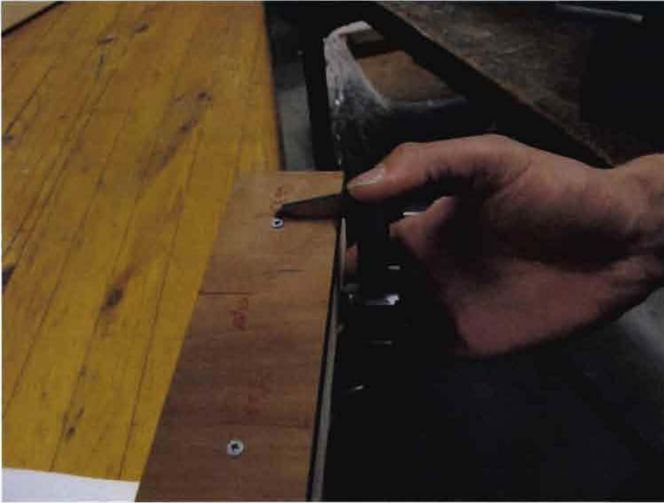
Figure 55: Measurement of adherent thickness before gluing
