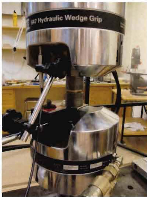
Figure 175: Tensile tests set-up.
