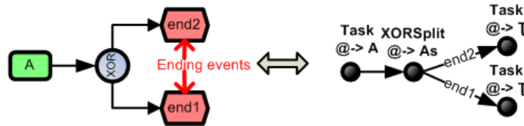
Figure 4.8: Canonical representation of an EPC model with 2 ending events following an XOR-split
