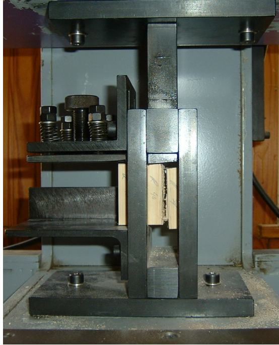
Figure 8.4: Test setup of block shear test
