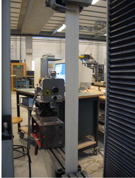
Figure 6.5: Test setup of tension test on single-layer laminations in combination with ESPI measurements
