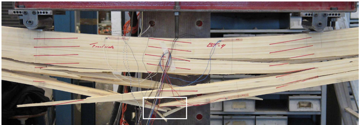
Figure 9.7: Failure of a laminated bamboo beam initiated at the scarf-joint
