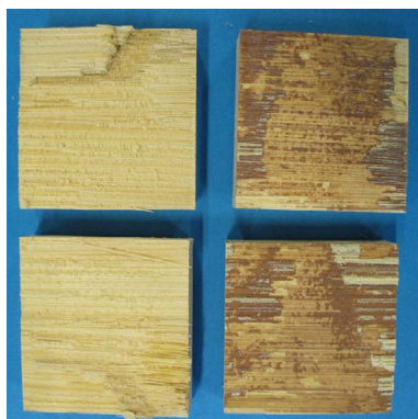
Figure 8.8: Bamboo failure: specimens of type MUF (left); specimens of type RP (right)
