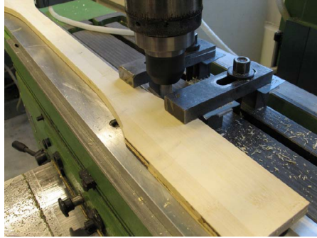
Figure 4.2: Reduction of the cross-section by using a milling-machine
