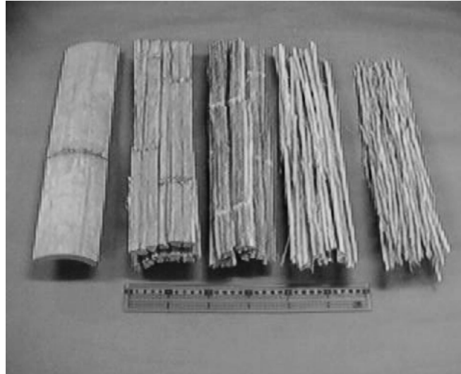
Figure 2.8: Bamboo zephyr strand from moso bamboo. From the left to the right side: bamboo culm, bamboo zephyr strands with diameter of 9.5 mm, 4.7 mm, 2.8 mm and 1.5 mm, respectively
