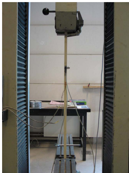
Figure 6.2: Test setup of tension test on strips
