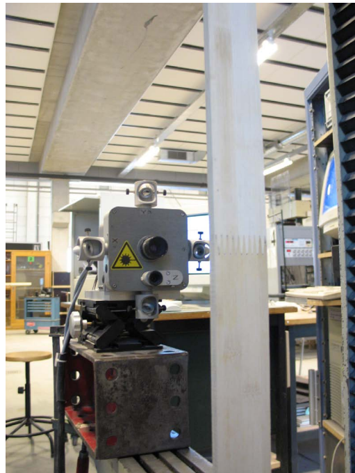
Figure 5.7: Test setup of tension test on finger-jointed triple-layer lamination in combination with ESPI measurements
