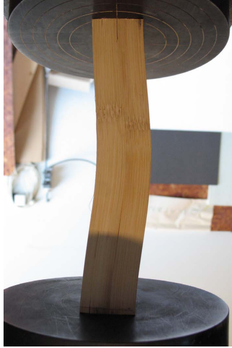
Figure 7.4: Failure initiated by buckling
