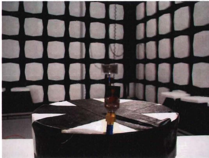
Figure D.2: Radiation pattern measurement with the antenna placed in the vertical position.
