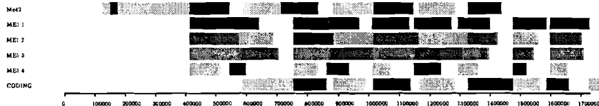
Figure 4.6: IMEC/MPSoC kernel execution schedule for QCIF resolution. On the vertical axis are the 6 processors, running respectively the ME42, four times ME1 and QC kernels.
