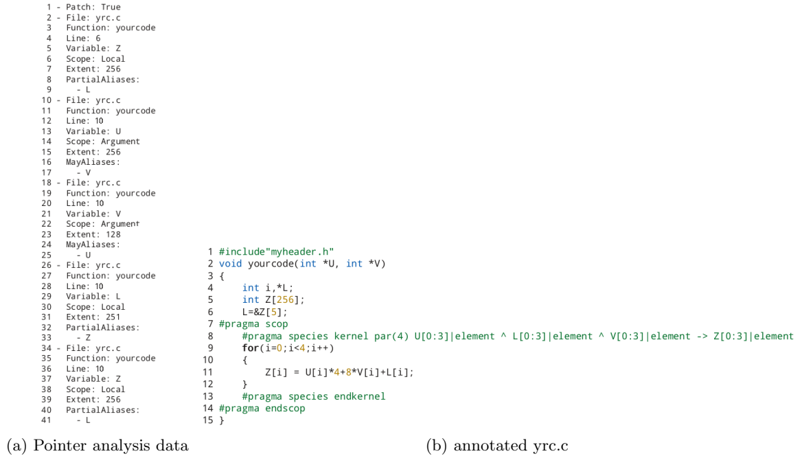
Figure 37: pointer analysis information for file yrc.c
