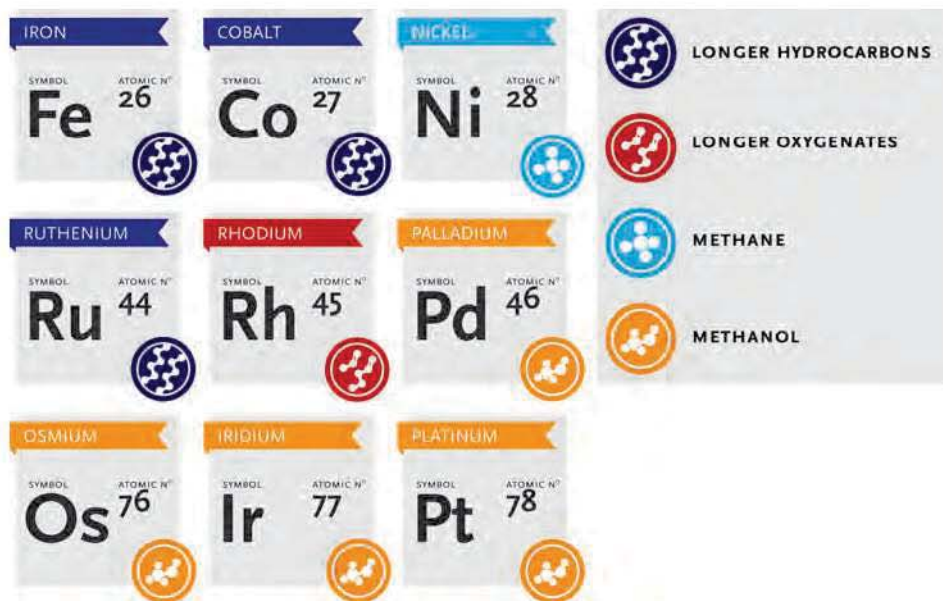
Figure 4: Different product selectivities with corresponding catalysts (by courtesy of Ir. Ivo A. W. Filot)
