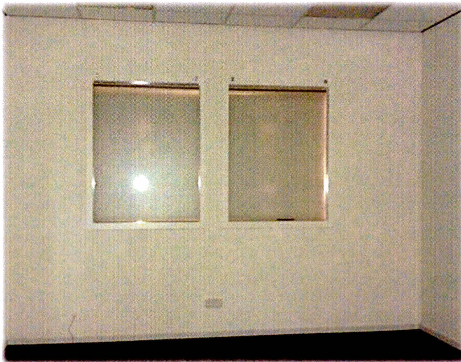
Figure 19 Virtual window structure observed from inside of the test room
