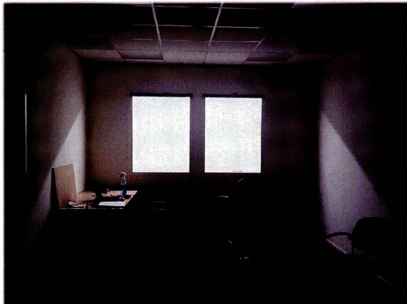
Figure 38 The direct light can create “sun patterns” on the sidewalls (iW Coves only)
