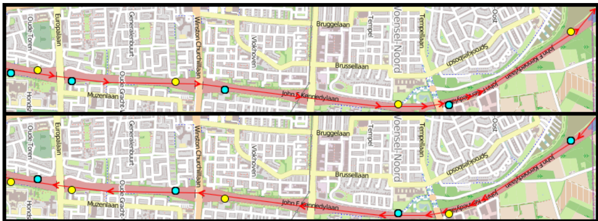
Figure 5.4: Measuring locations linked to John F. Kennedylaan . The arrows on the road show the traffic direction and the dots in blue indicate the locations that measure the traffic in that direction.
