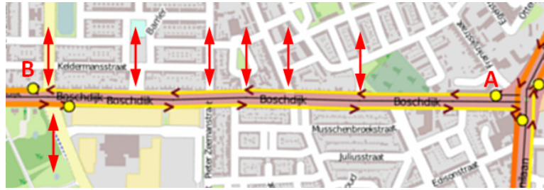
Figure 5.18: Traffic intensity of " >5.6m <12.2m " vehicle class on a section of Boschdijk street. The red double arrows show the possible entrance-exit locations for the traffic on the top lane (going left) between measuring locations A and B.
