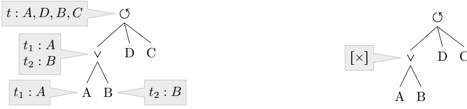
(a) Process tree in which the alignment of Figure 5.7a is mapped onto the nodes and partitioned for the children of the loop construct.
