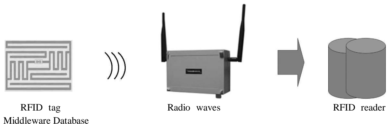
Figure A.1: The basic elements of RFID technology are tags, readers, and middleware
