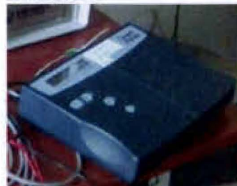
Figure: 2 dataloggers (1 to logg lamp on/off (ID 1816, serial port, 1F8), and 1 (ID 1815, usb, 2F8) to logg CO2, air-velocity, ambient air temperature, relative humidity and radiant temperature)
