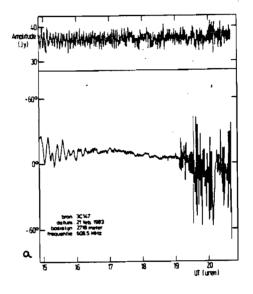
Ionospheric irregularities observed on a baseline of 2.7 kilometer. The top figure shows the interferometer amplitude and the lower the phase as a function of time. During the first 1  $\frac{1}{2}$  hours, slow wave phenomena distort the measurements and after 2  $\frac{1}{2}$  hours of quiet conditions the last part is distorted by fast irregularities.
