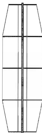
Figure 3.3 A glass-steel column consisting of a number of small glass panes, instead of one large pane, allows for higher material efficiency and better possibilities to ensure residual load capacity upon breakage of one or more panes.
