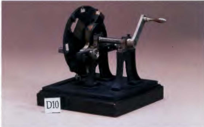
A reciprocator or ellipsograph, transforming axial movement into oval movement (source: wikimedia)
