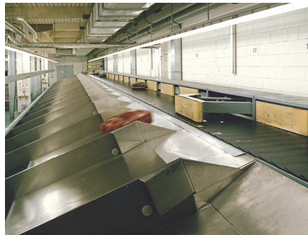
Figure 11: A flat Triplanar carousel with Divert Parallel Pushers and chutes (Vanderlande Industries, 2010)
