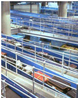
Figure 10: A lane storage system (Vanderlande Industries, 2009d)
