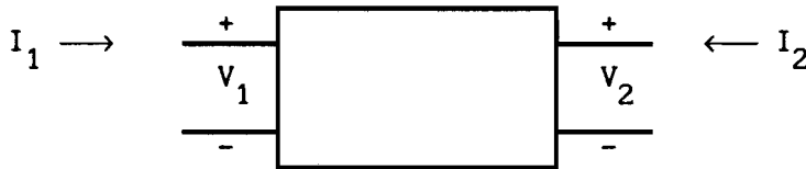
Fig. 4.7 : Two port representation of circularly polarized microstrip antenna for calculation of the input impedance.
