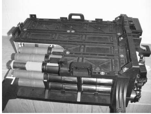
Figure 2.8: The battery pack of the Honda Civic IMA
