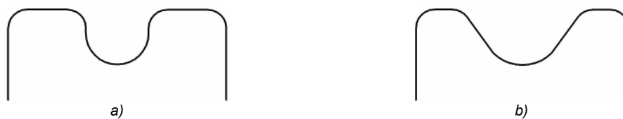
Fig. E.5. a) Initial roller groove shape. b) Proposed adjusted roller groove shape.
