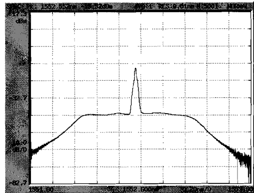
Figure 6.4: Spectrum of the modulated signal. The carrier and the filtering can clearly be distinguished.
