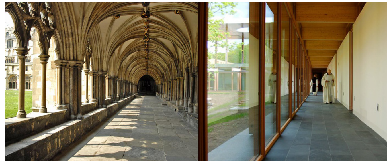
fig. 25 & 26 Norwich Cathedral (1145) in Norwich, UK; Val Notre-Dame Abbey (2010) by Atelier Pierre Thibault in Saint-Jean-de-Matha, Quebec, Canada. Cloisters are characterized by a number of recurring elements. Orientation is one-sided, with one closed wall and one open, with a view to a garden. The open wall is very rhythmic, creating a rhythm in the corridor and a sequential view outside. The end of the cloister is often closed. The end can be dark or lighter, clearly visible as the end, but without it being clear what goes on beyond the corridor. This creates a notion of endlessness, the cloister always seems to continue around the corner.
