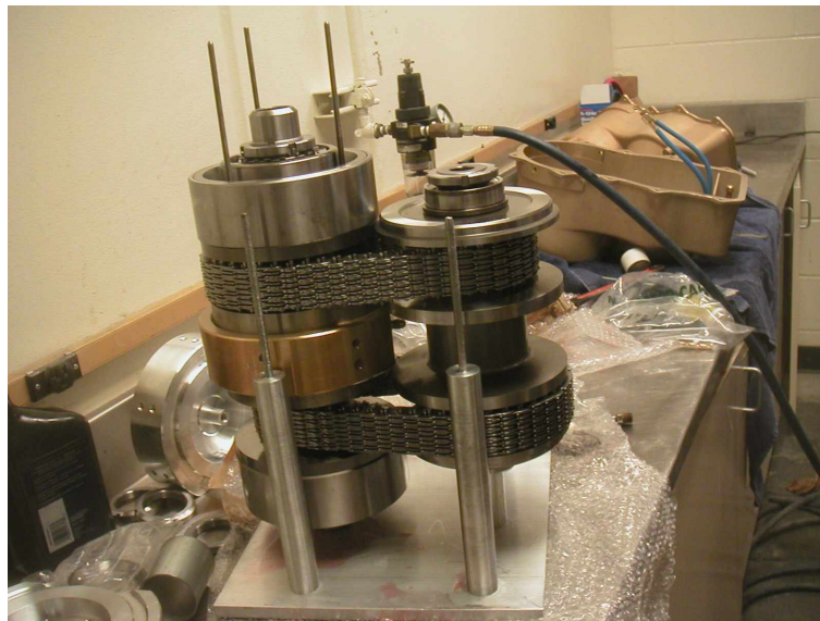
Figure 2.4: The bracket to assemble the CVT
