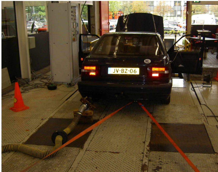
Figure 4.18: The Volvo 440 at the dynamometer to tune the pressure- and ratio controller.
