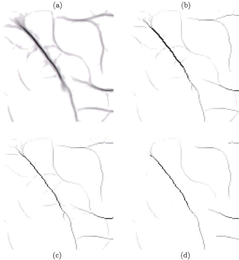
Figure 5.4: Example of thinning. (a) Input image R (result of tensor voting). (b) Result after thinning. Only the centerlines are kept. (c) Result after skeletization. (d) Result after 14 pruning steps. The colors of all images are inverted.
