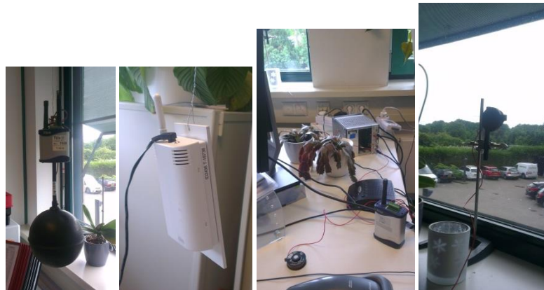
Figure 61: From left to right; measurement positions, black globe temperature and humidity measurement equipment, CO 2 temperature and humidity measurement equipment, illuminance measurement equipment on the desk, illuminance measurement equipment in front of the window.
