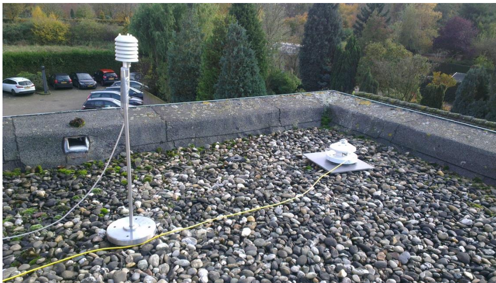
Figure 72: On the left in the picture temperature and humidity measurement equipment and on the right the pyranometer.
