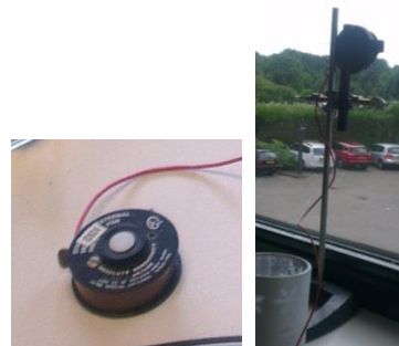
Figure 15: Illuminance detectors, left at the desk right in front of the window.
