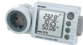
Figure 18: Applied Voltcraft energy logger 4000, logging electrical appliance load at the workplace.
