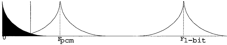
Figure 3.1: Spectral folding around \frac{1}{2}f_{pcm} of error-components which lay outside the PCM-band when the filtered 1-bit signal is sub-sampled to the PCM sampling-rate.
