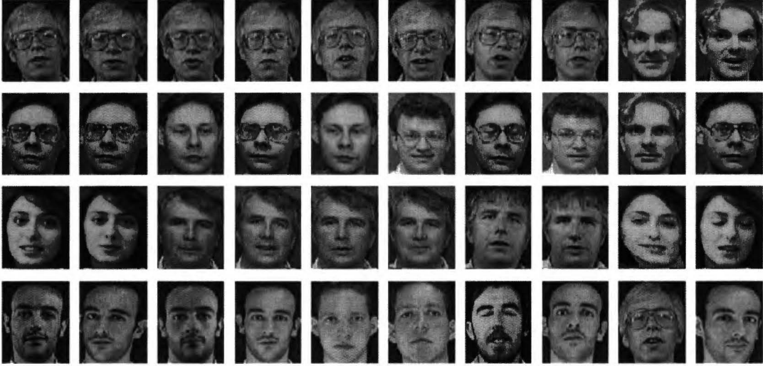
Figure 5.1: Experiment 1: d_{ij} = \sqrt{(x_i - x_j)^2 + (y_i - y_j)^2 + (t_i - t_j)^2} and weights are equally distributed. Leftmost images are queries, neighboring images are closest matches, with increasing PTD.
