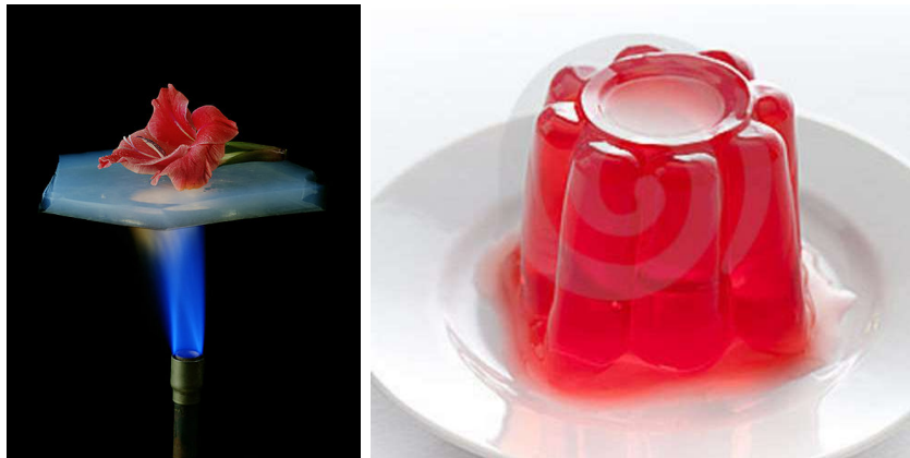
Figure 1.2: An aerogel functioning as isolation between a flame and a flower (left). A typical example of a strong physical gel we all know, gelatin (right).
