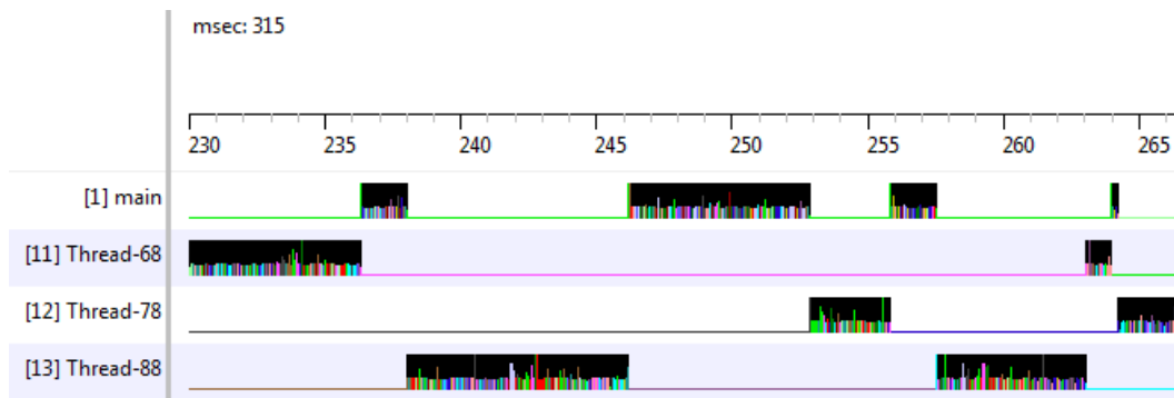
Figure 17: Trace view of the scalability test 3. [11] Thread-68, [12] Thread-78 and [13] Thread-88 show the Shimmer threads that are handling the Bluetooth connections.
