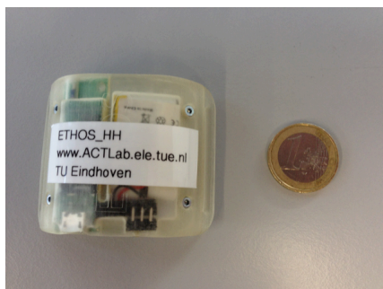
Figure 13: ETHOS attitude heading and reference system.
