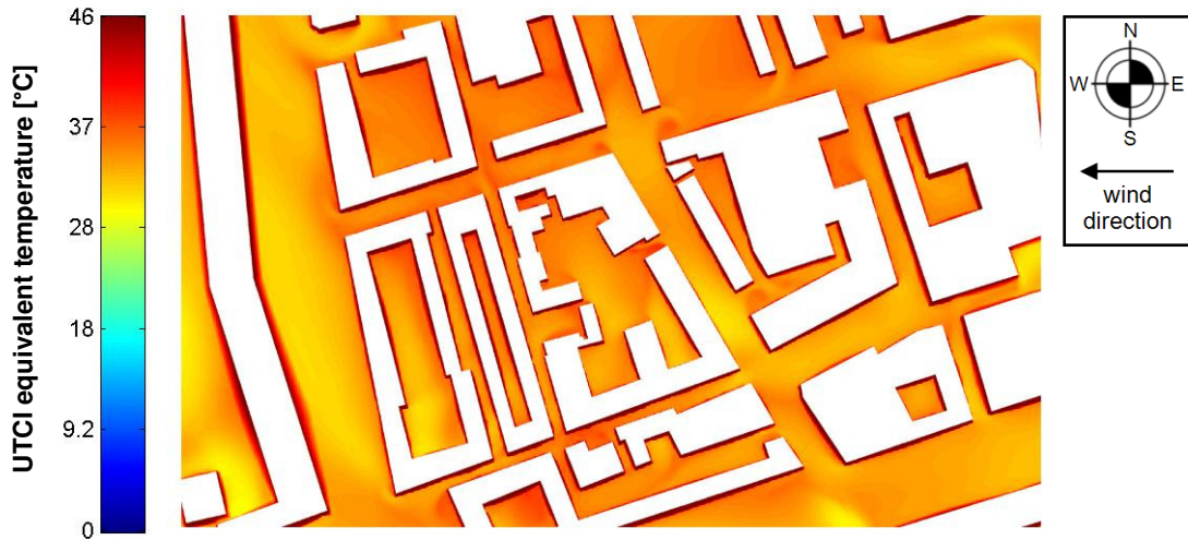
Figure 6.18: UTCI equivalent temperature [°C] around the care center at 17 July 2006, 11:44 am
