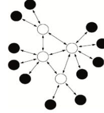
Figure 9: Hybrid Star-Mesh Topology Source: (Matin & Islam, 2012, p. 9)
