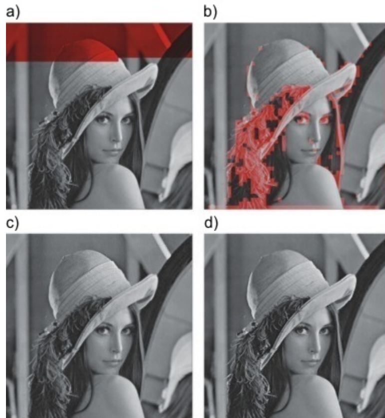
• Figure 3: Example result of applying an scalable sharpness enhancement algorithm: a) The blocks of the image are processed in sequential order; b) The most important picture parts are identified and processed. In both images the red parts show the progress of the algorithm. c) The result of the sequential algorithm in which only background content is filtered and therefore no visible quality improvement is obtained. d) The result of the priority processing algorithm when the most important image parts are enhanced. Source: [6]
