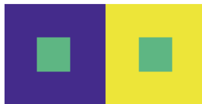
Fig. 2-6 Simultaneous contrast. The green square appears different when viewed with different surroundings.
