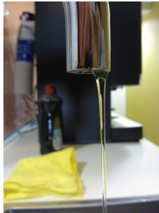
Figure 2.2.6: Our own experiment with an every day realization of surface tension: we photograph running tap water to measure the diameter at different heights and collect the water to measure the average flow rate.
