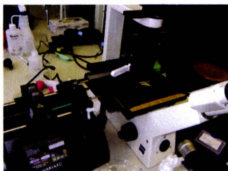
Figure E.1: The left image shows the experimental setup. To the left is the syringe pump, on which lies the syringe. A blunt needle connects the syringe to the tubing going into the device placed on the microscope. The right image shows a sealing clip, used to block tubing.
