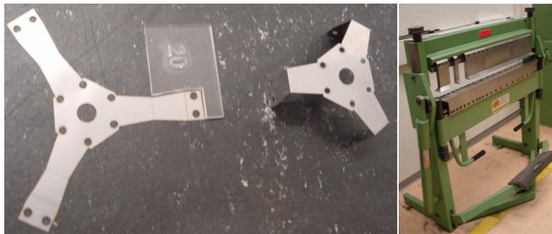
Figure 3.17: folding the leaf springs, left an unfolded and folded leaf spring membrane, right the bending machine.
