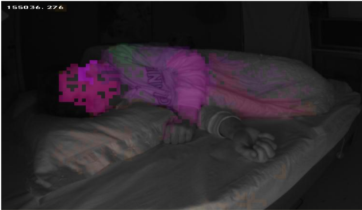
Figure 19: Motion vectors after propagation elimination. The detected motion vectors specify the true motion with higher accuracy.
