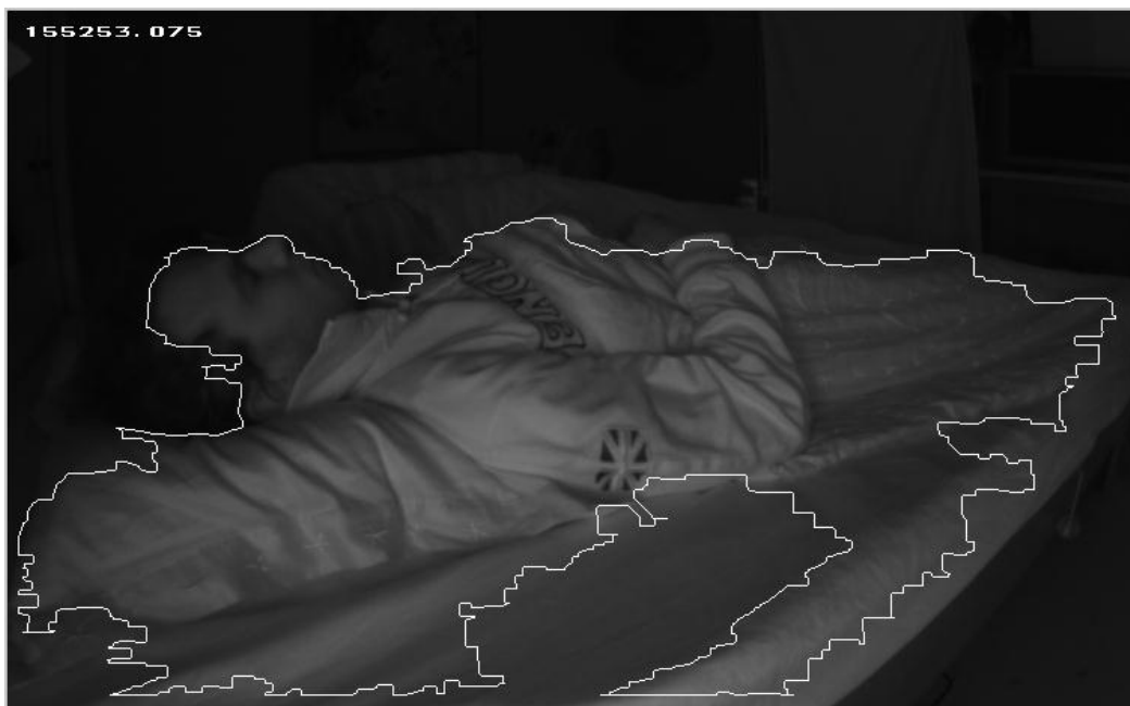
Figure 14: Intermediate output with all closed regions as a result of region filling.
