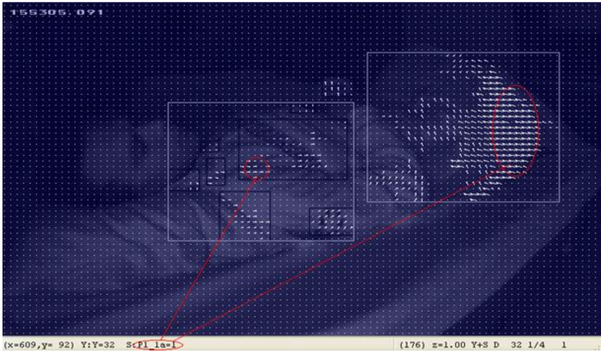
Figure 23: The assignment of motion blocks to POI and BP after adding the spatial constraint. Label 1 (seen as P I_la =1 in the image) indicates that the motion rectangles (seen as white rectangles) are assigned to POI.
