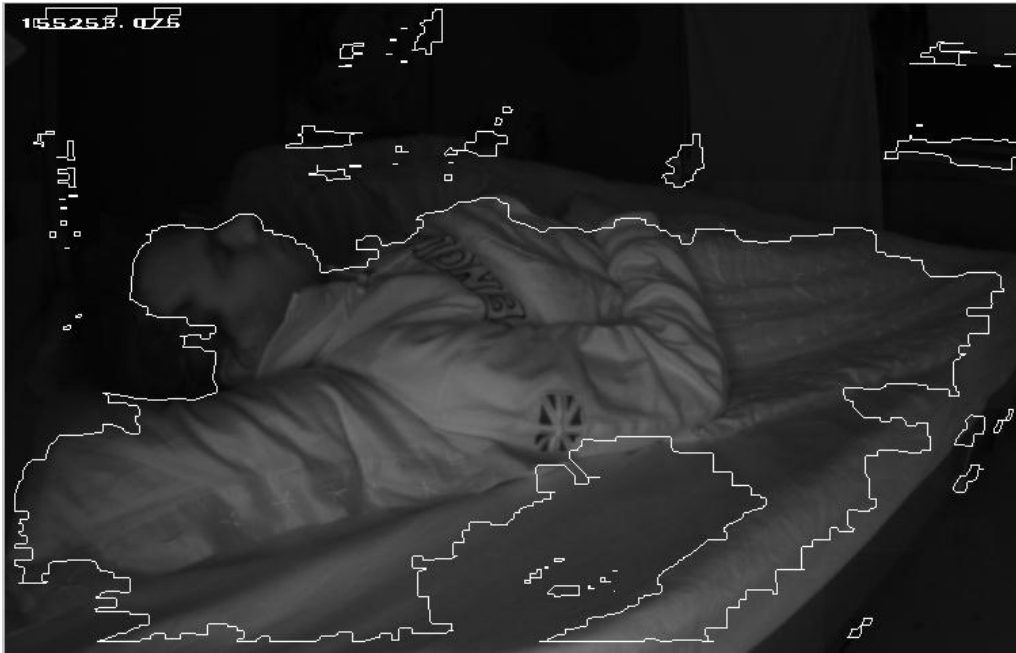
Figure 14: Intermediate output with all closed regions as a result of region filling.
