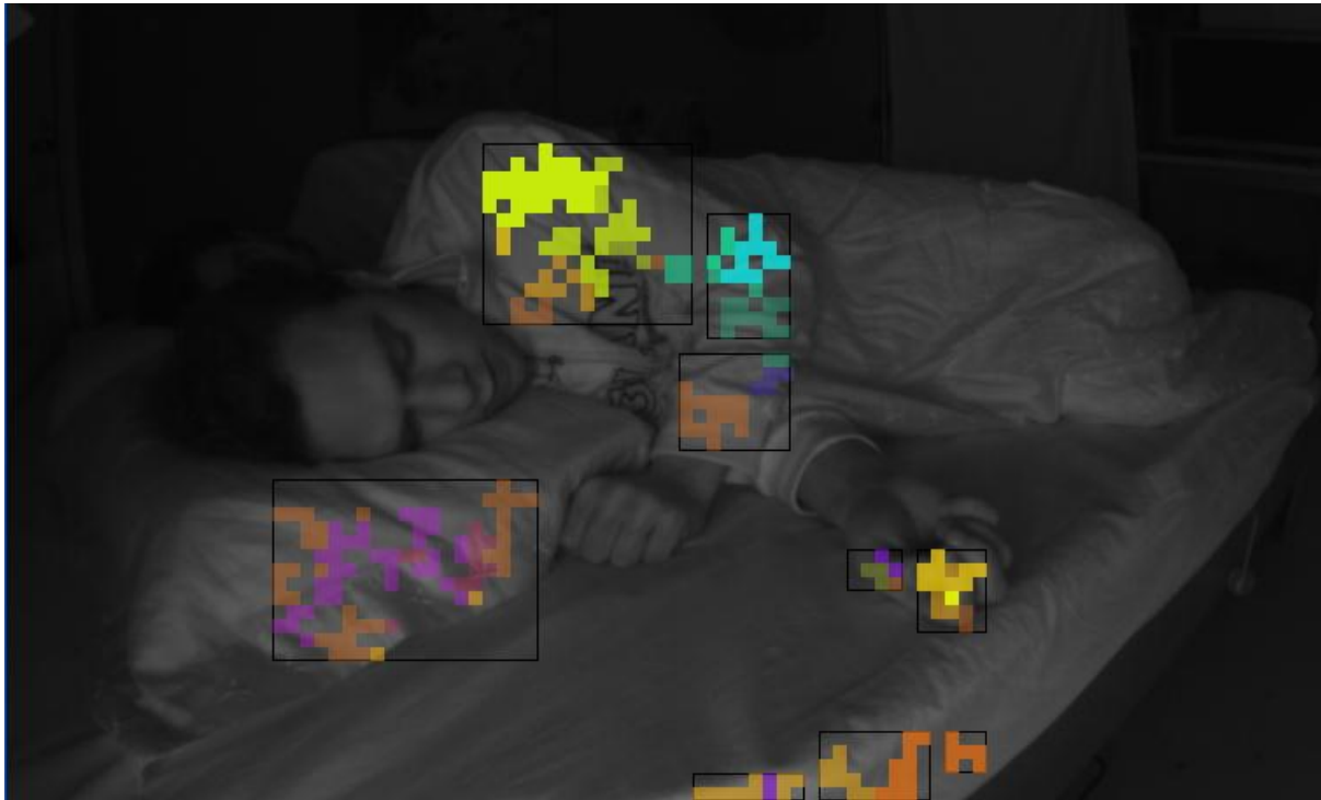
Figure 21: Generated motion rectangles containing motion blocks (seen in colours).
