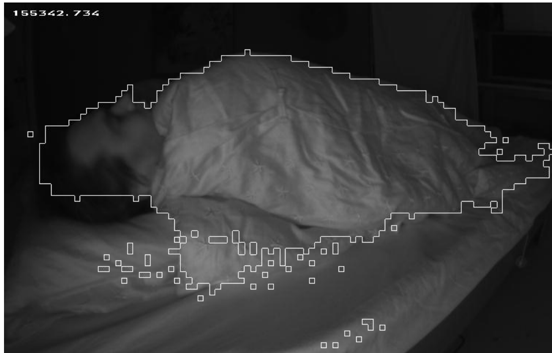
Figure 32: AdaBoost classified output of POI segmentation result. The closed regions given by the white line show the classified POI area in the image.
