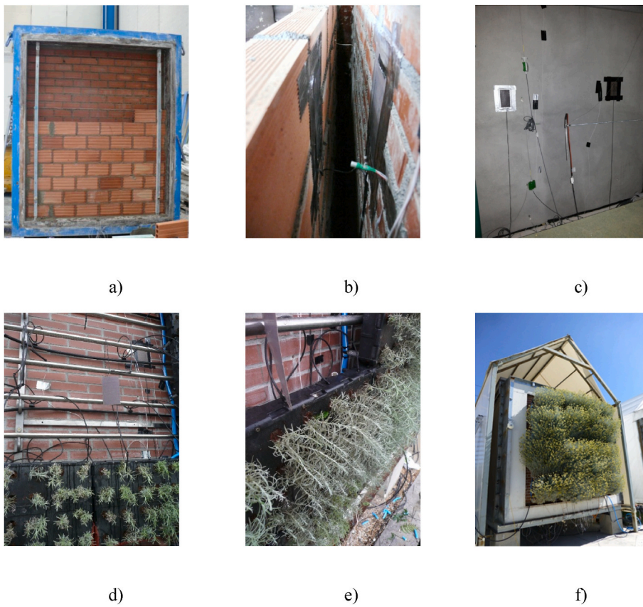
Fig. 5. Details and measurement devices of the constructive system in the experimental setup in the PASLINK test cell. Above: a) Base wall (BW) detail of the double hollow brick and the perforated brick. b) detail of the sensors and their position in Layer 3, the air chamber. c) detail of the sensors in Layer 1, the internal part of the surface 1. Bottom: d) The MLW of the experimental set up with modular metallic sub-structure and sensor positions. e) detail of the irrigation system and the modular pots with vegetation. f) Experimental set-up of the MLW in Vitoria-Gasteiz, Spain.
