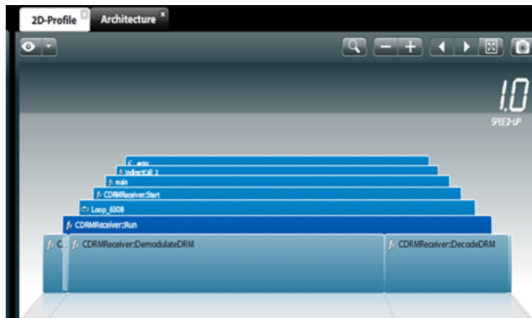
Figure 5.14: The Pareon's function distribution of the DRM program
