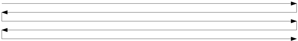
Figure 3.10: Zig-zag scanning pattern.
