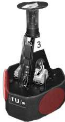
Figure 1.1: Surfaces of the Turtle used for pushing are indicated in red [8].
