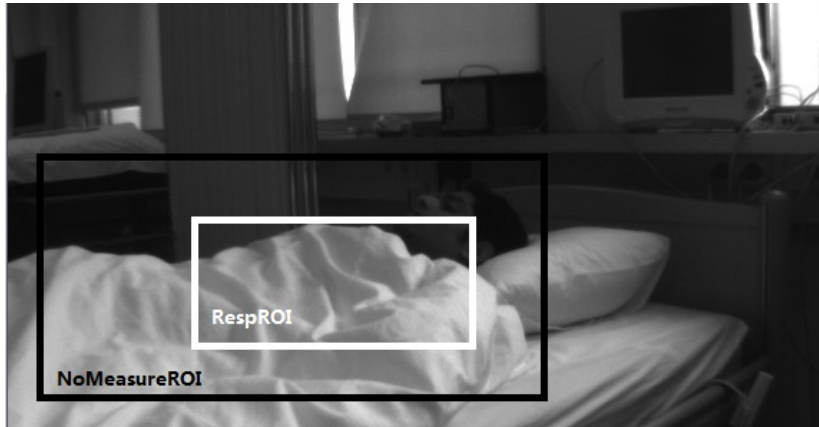
Figure 2.1: RespROI and NoMeasureROI displayed in the frame: the white rectangle is RespROI, as the original input of respiration measurement algorithm(ProCor). The black rectangle is NoMeasureROI, input of the compensation algorithm proposed by van den Helder [27]
