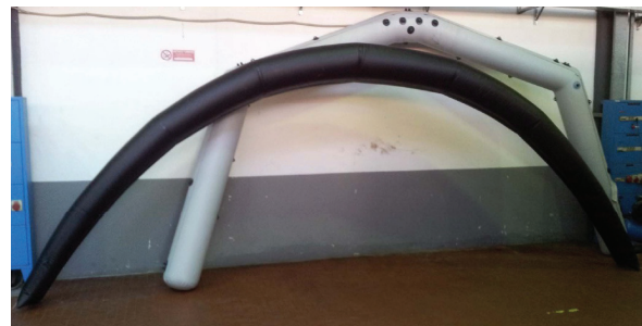
Figure 3.19: Prototypes of tensairity arches by Roberto Maffei (Maffei 2013)
