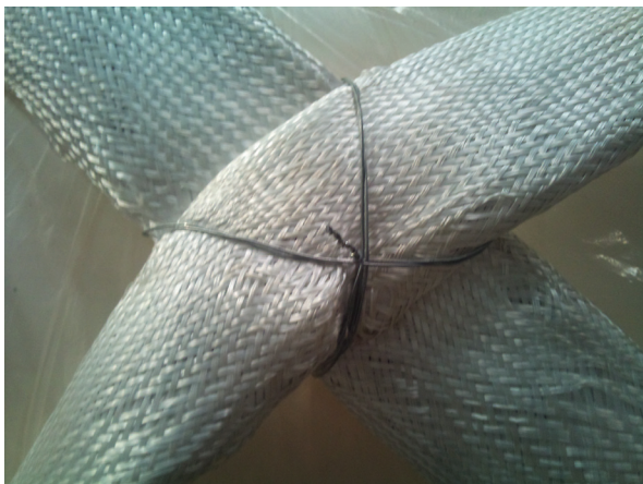
Figure 8.8: Junction between two fire hoses
