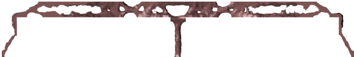
Figure 2.41: Multipanel frame with a point load
