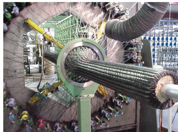
Figure 3.38: The (over)braiding process of Eurocarbon B.V.
