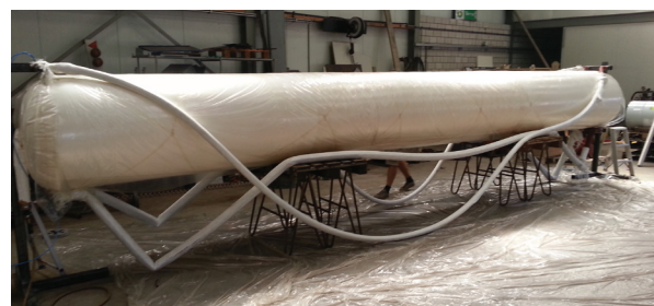
Figure 8.4: Inflated unfixed fire hoses with double glass fibre biaxial weave
