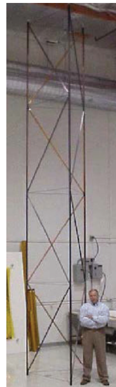
Figure 4.17: SOTC with shape memory truss (Guidanean & Lichodziejewski 2002)
