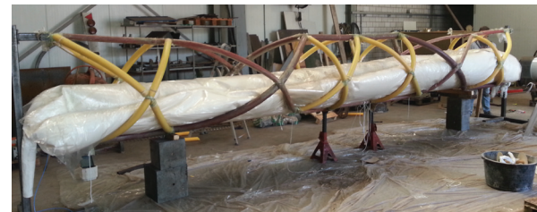
Figure 8.8: Deflation of the secondary mould
