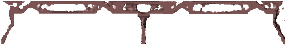
Figure 2.40: Multipanel frame with a distributed load
