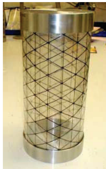
Figure 4.22: Sample of an UV cured composite by ILC Dover inc. (Allred et al. 2002)
