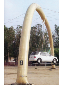
Figure 3.15: Inflatable arch by the U.S. Army for temporary shelters.
