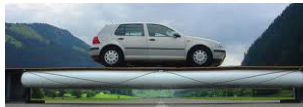
Figure 3.18: TOP; Basic elements of Tensairity (Luchsinger et al.) BOTTOM; Tensairity beam (Airlight Ltd.)
