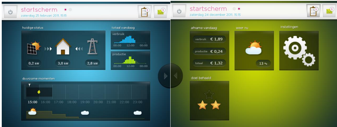
Left: Homescreen showing the current electricity consumption, production, totals of today and prediction of beneficial electricity usage moments. Right: 2 nd Home screen with total costs of usage, total benefits from production, the current weather forecast, settings and reached goals.
