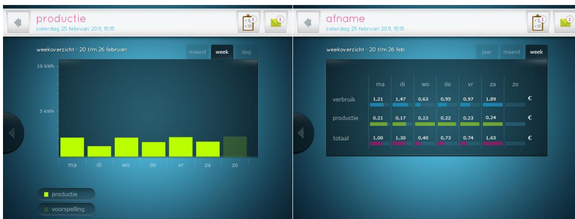
Left: Production screen with weekly production and forecast. Right: Financial overview showing weekly consumption costs and production benefits.
