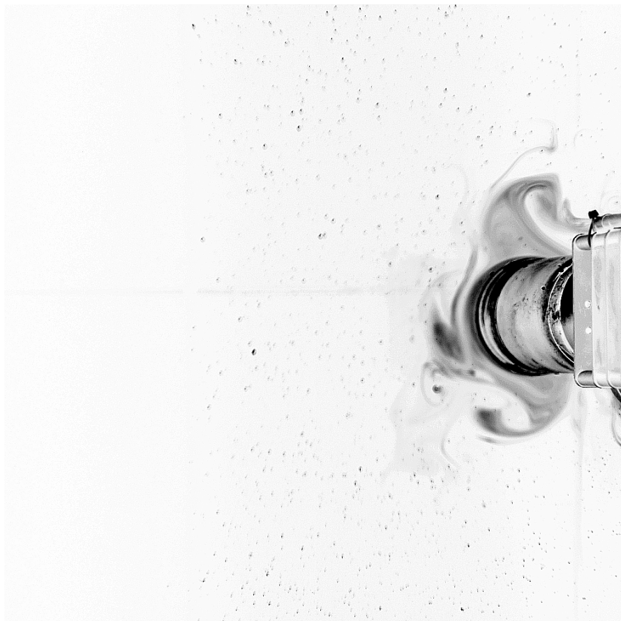
Figure 5.3.: Typical result of the rotating table setup in which the cylinder has rotated for 20 s. The picture is taken 50 s after impulsively halting the cylinder. An instability has occurred, but no coherent structures can be distinguished in the dye around the cylinder.
