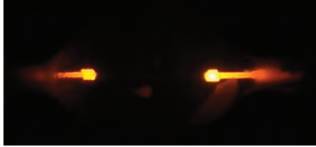
Figure 4.4 The figure shows the electrodes of a lamp shortly after extinction. Switch-off measurements will group electrode radiation with the thermal radiation of the burner wall. This is separated by extrapolating the switch-off data.
