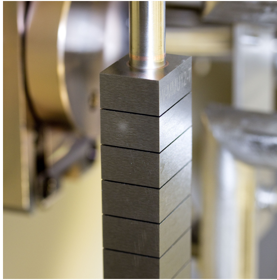
Figure 5.6: Photograph of the ITER-monoblocks after exposure to 17400 plasma pulses and 88 shots in Magnum-PSI. The plasma-wetted tile shows a white spot indicating an increase of emissivity.
