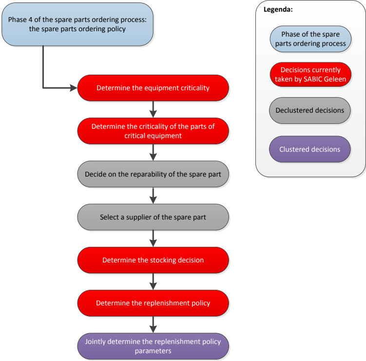
Figure 2: adjustments of the decisions and sequence of the spare parts ordering policy
