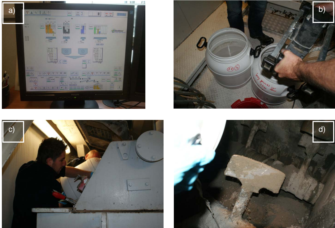
Figure 6-3; a) Automatic weight system, b) dispersion by a hand concrete mixer, c) adding nSS into the mixer, d) nSS in the mixer
