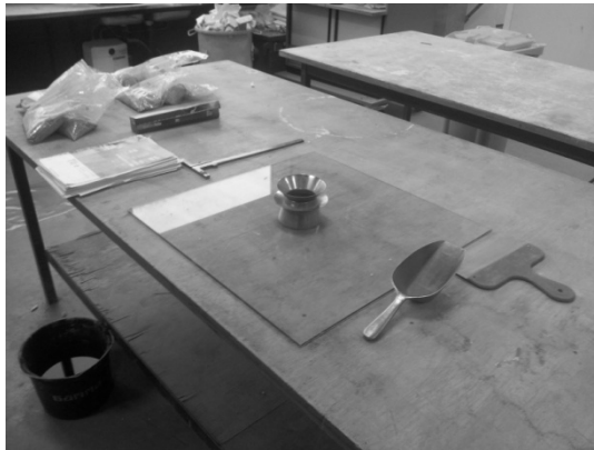
Figure 5-1; Hägermann cone test setup (Source; picture J van der Putten)
