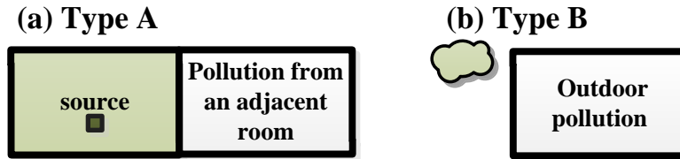
Figure 41: The pollution types which are considered during this study: Type a is located indoors while type b originates from outdoors and is the default pollution type used in this study. Note that both sources are external sources.
