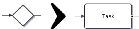
Figure 6.8: Gateways with an in- and outdegree of one can be transformed to a task node.
